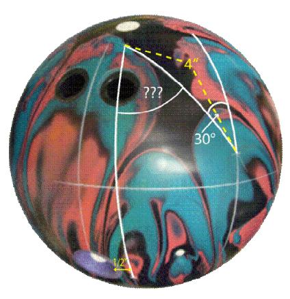
On an existing ball, draw a 30° angle to the VAL. Place the Pin 4" from the **PAP** on the 30° angle line. Draw the base line to pass ½" to the right of the thumb (½" from the outer sleeve of a Switch Grip). Measure the **drilling angle** to be used as it will be different for every **PAP**.
