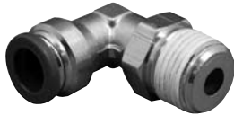
11655040000 Fitting - 3/8" Dia. Tube Prestolok to 3/8" NPT, 90° Swivel Used on Injector Rail, Accumulator Rail, and Cleaner Manifold
