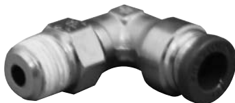
11655017000 Fitting 1/4" Tube, Prestolok to 1/8" NPT, 90° Swivel Used on Conditioner Pressure Control Valve
