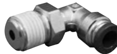
11655026000 Fitting 1/4" Tube, Prestolok to 1/4" NPT, 90° Swivel Used on Conditioner Tank and Plastic Filter
